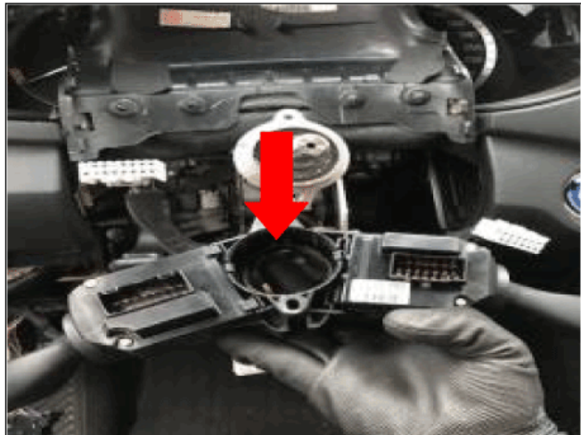
Multifunction switch noise Replace multifunction switch
