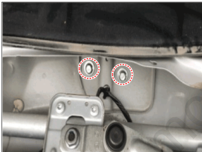
Cowl top bolt mount defect Retighten cowl top bolt
